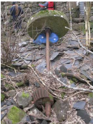
Millstone attached to iron driving rod and toothed gear.
